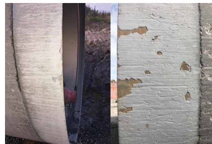
Figure 5. Epoxy Coated Bell Ring After Drive.
