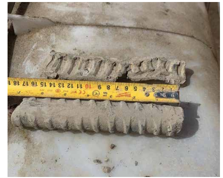
Figure 10. Tie Back Recovered in Slurry Pump.
